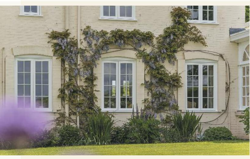
Cottage casement windows finished in 'White', with 18mm astragal glazing bars. Manufactured in Engineered Meranti Hardwood.
