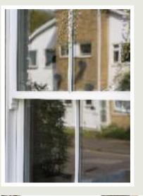
Slim sash windows in "White" with traditional horns to upper and lower sashes, 18mm astragal bars, and hung on a cords and weights mechanism are accompanied by a also in "White" with
