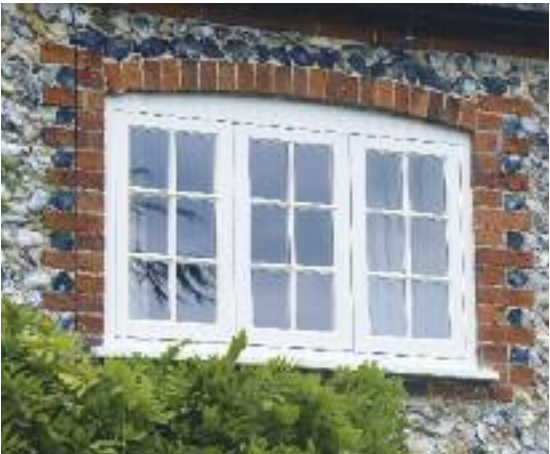
Cottage flush casement windows finished in “Off-White” featuring 24mm true bars, putty glazing and 14mm ultra slim double-glazed units.
