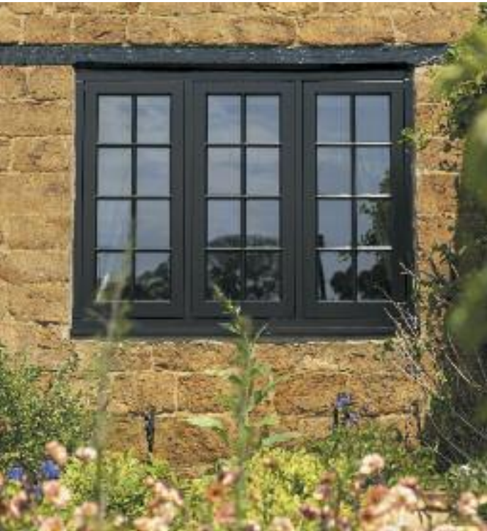
Flush casement windows finished in ‘Black’ with 14mm ultra-slim double-glazing, putty finishing, 24mm true bars, and Antique Pewter Monkeytail handles and pegstays.
