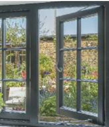
Flush casement windows finished in ‘Black’ with 14mm ultra-slim double-glazing, putty finishing, 24mm true bars, and Antique Pewter Monkeytail handles and pegstays.
