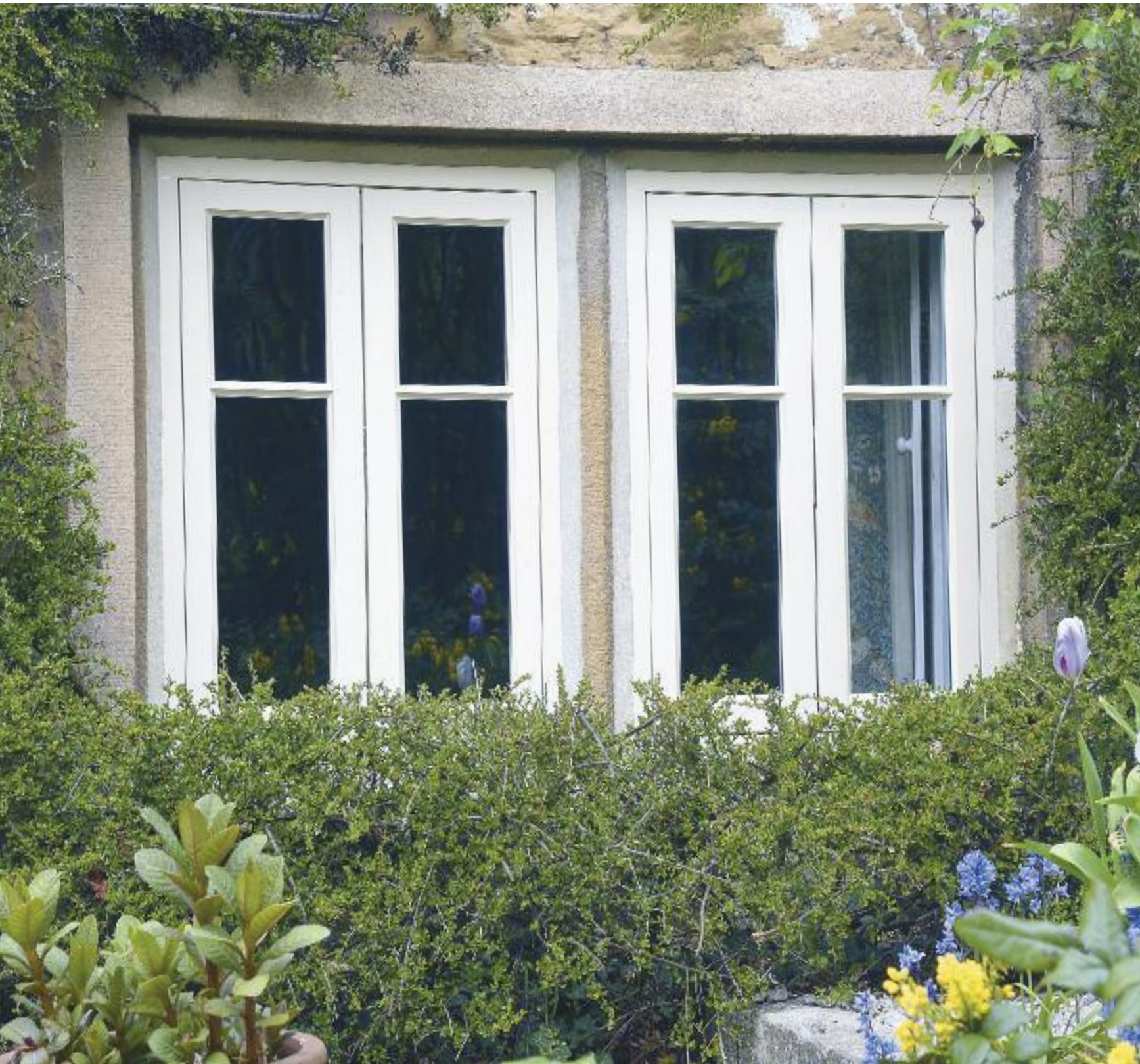
Cottage flush casement windows featuring 14mm ultra slim double glazed units with krypton gas, 24mm true bars and putty glazing, externally finished in the shade of 'Dorset Cream' and internally in 'White'.
