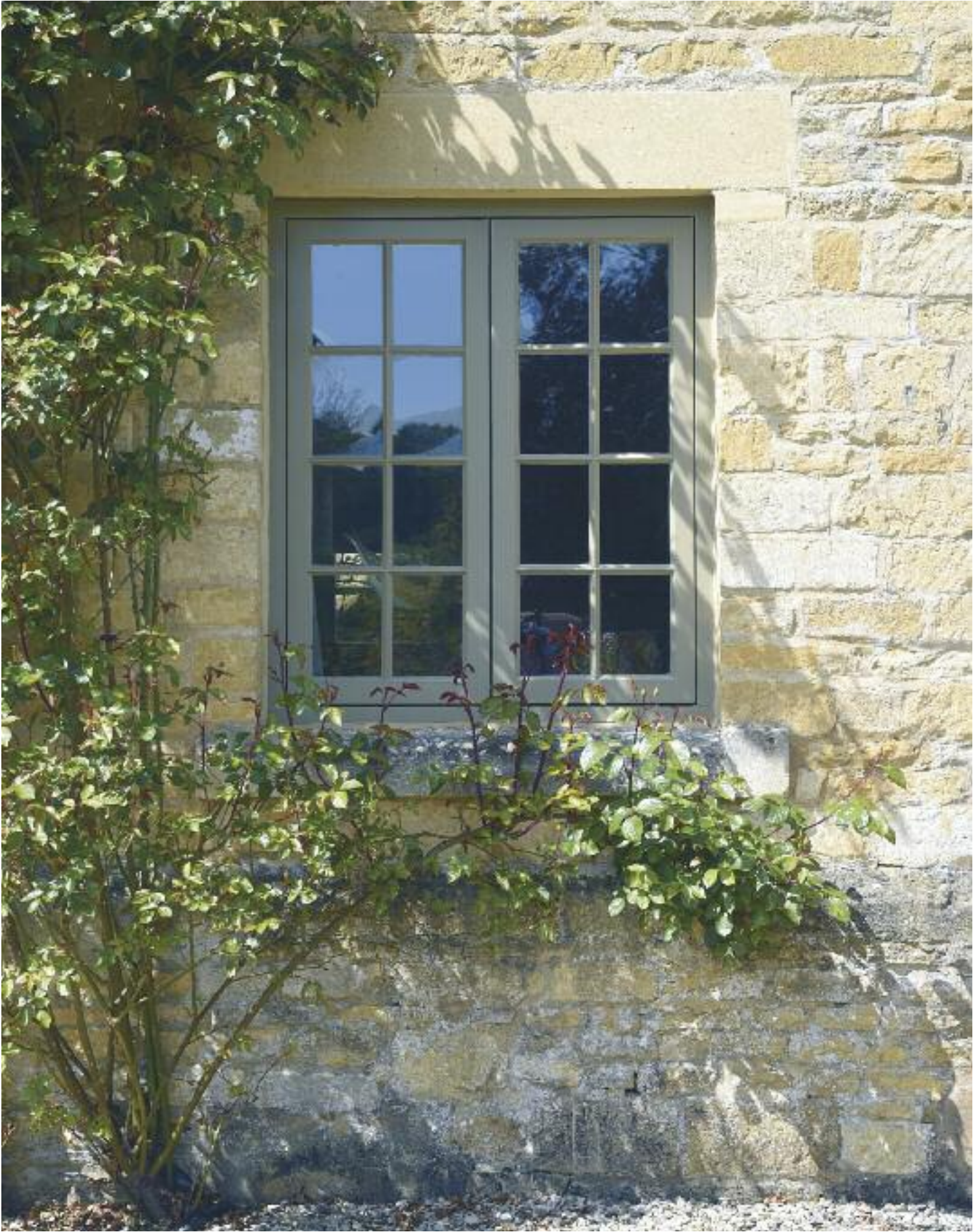
Cottage flush casement windows in the shade of 'Oxide Gold' externally and 'Off-White' internally with 24mm true bars, putty glazed and 14mm ultra slim double glazed units.
