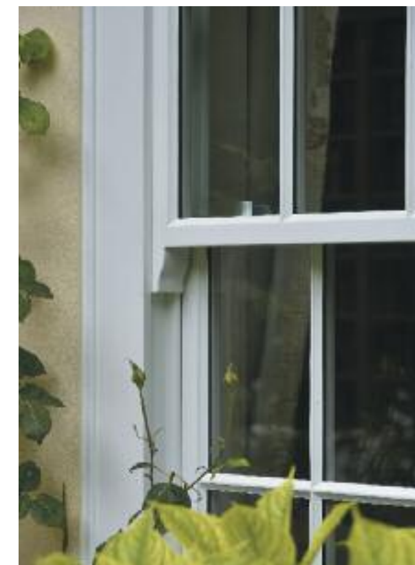
Slim sash windows hung on traditional cords and weights mechanisms, finished in White with 14mm ultra slim, putty finished double-glazed units and 24mm true bars.
