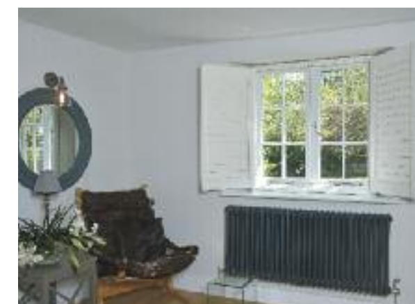
Cottage flush casement windows, finished in 'White' with 4mm single putty glazing. 24mm true bars manufactured in Engineered European Redwood (14mm ultra slim double glazing to rear property windows)
